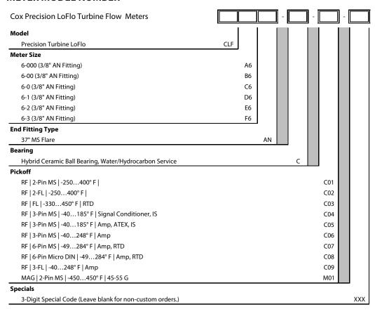
Turbine Flow Meters, Precision Series LoFlo Meters
